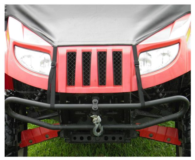
Wrap these straps around the bumper and thread the end of the strap through the clip. Pull straps tight.
