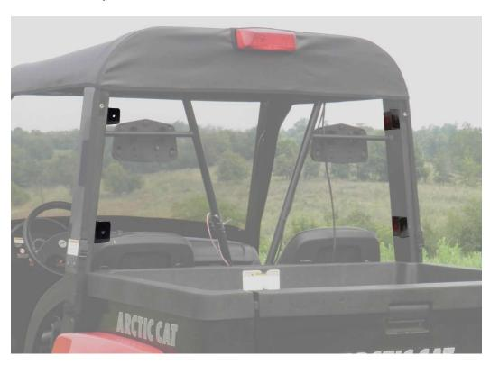
**Step 3:** Each side of the Back Panel requires 2 clamps, bolts, neoprene washers, small washers, and lock nuts. Prepare the bolts for use by inserting the bolt through the neoprene washer and sliding it on so that it sits against the head of the bolt.
