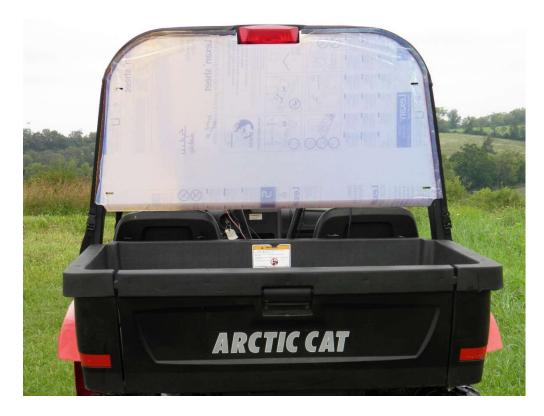
**Step 6:** When satisfied that the Back Panel is positioned properly, tighten the lock nuts.
