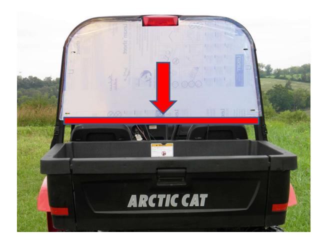
**Step 8:** Raise the bed of the UTV and attach the 18" pieces of velcro down each side of the roll bar to align with the sewn-in velcro on the outer edges of the lower back panel
