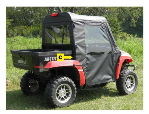
**Step 3:** If not already done, drape the windshield/top combo over the roll bars. Align the windshield/top square to the roll bars. Begin attaching the sewn-in loop strips to the adhesive hook strips as indicated in the tables above.
