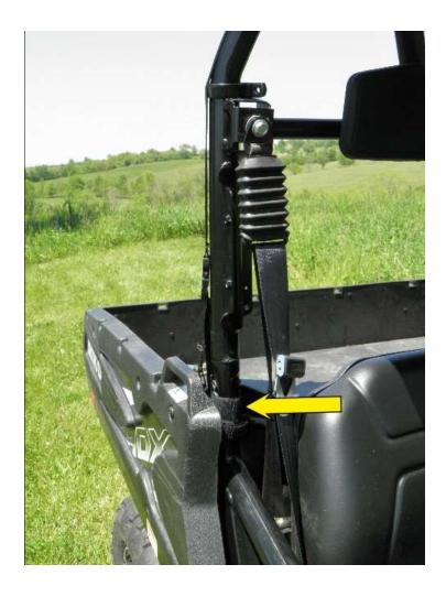
**Step 5:** Wrap the sewn-in double-sided straps at the bottom of the tension strap around the adhesive hook strips. If needed, loosen the tension strap to extend the length of the strap. DO NOT PULL TIGHT AT THIS TIME.
