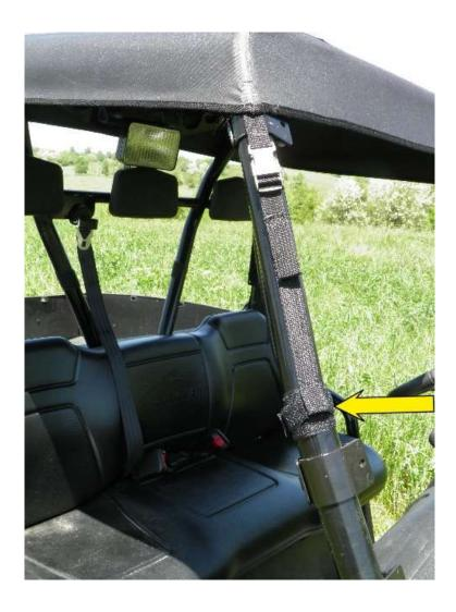
**Step 7:** Wrap the sewn-in double-sided straps at the bottom of the tension strap around the adhesive hook strips. If needed, loosen the tension strap to extend the length of the strap. DO NOT PULL TIGHT AT THIS TIME.
