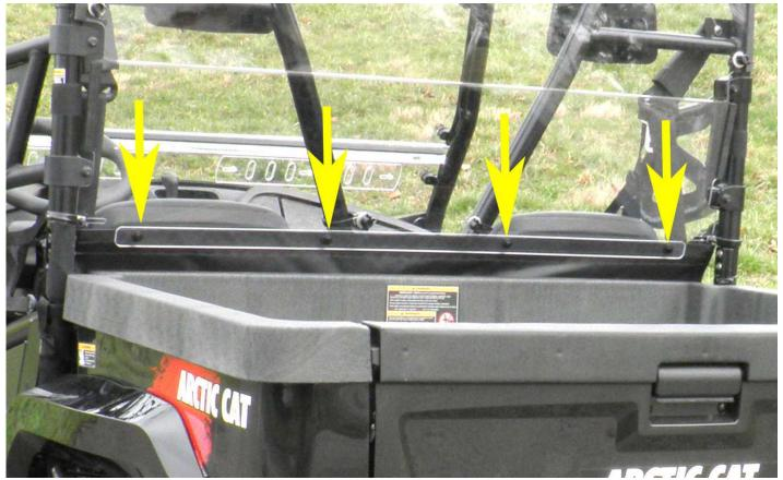
Step 6: Line the grommets on the fabric panel up with the slots in the lexan back panel. Sandwich
