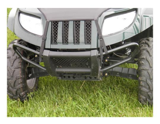
The double-sided velcro at the bottom of the straps on the back corners of the windshield/top wrap around the 6" velcro strips that were installed on the roll bars.
