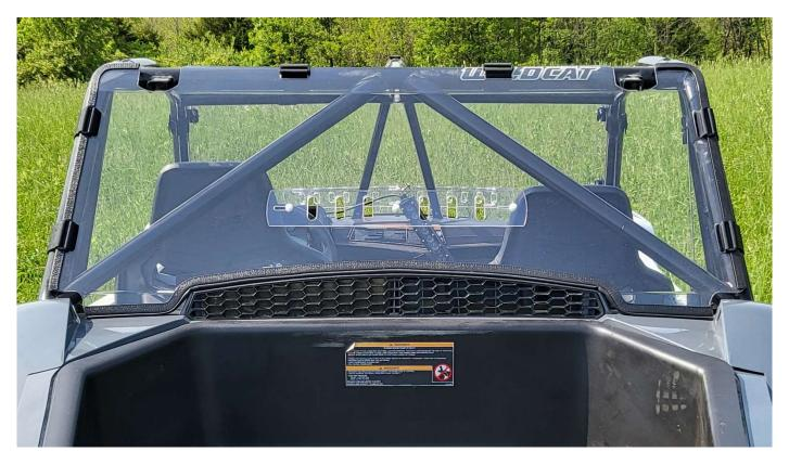
Set back panel on the roll cage. Peel back the paper to expose the pre-cut slots. Insert strap through the outside of the windshield, wrap around the bar, insert end of strap through plastic buckle, pull tight and connect hook to loop. Repeat for all remaining straps.
