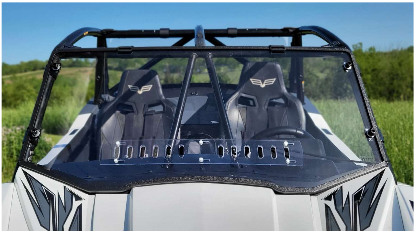
Figure 2.1 - Center Windshield between roll bar so that edges are in the center of the front Roll Bar posts
