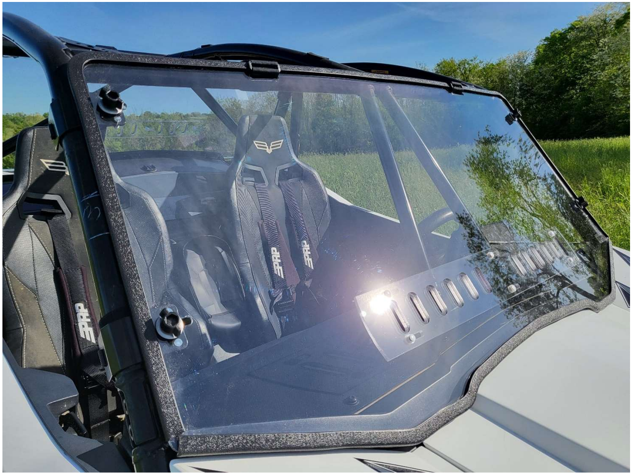
Figure 2.1 - Center Windshield between roll bar so that edges are in the center of the front Roll Bar posts
