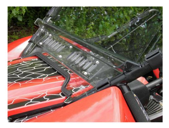
**Step 6:** Repeat Step 4 for each of the strap slots in the upper windshield section.
