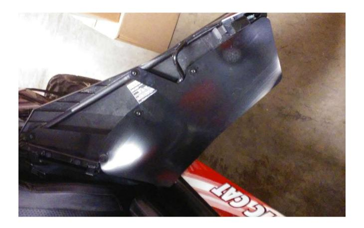
**Step 3:** line the door kits slot holes up with the factory drilled holes in the door frame.
