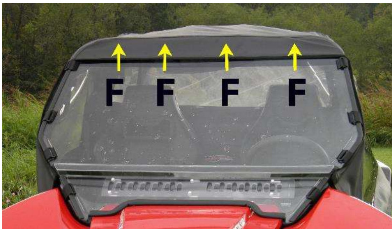
Figure 5: Photo shows placement of Velcro strips F. place strips on the underside of the roll bar. Pull tabs over the top of the roll bars and attach to the underside of the roll bar.
