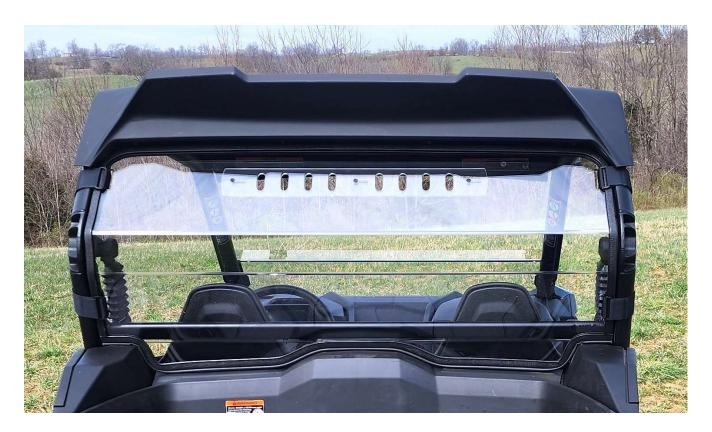
Set windshield in the pro-fit track. Peel back the paper to expose the pre-cut slots. Insert strap through the outside of the windshield, wrap around the bar, insert end of strap through plastic buckle and pull tight. Repeat for all remaining straps.
