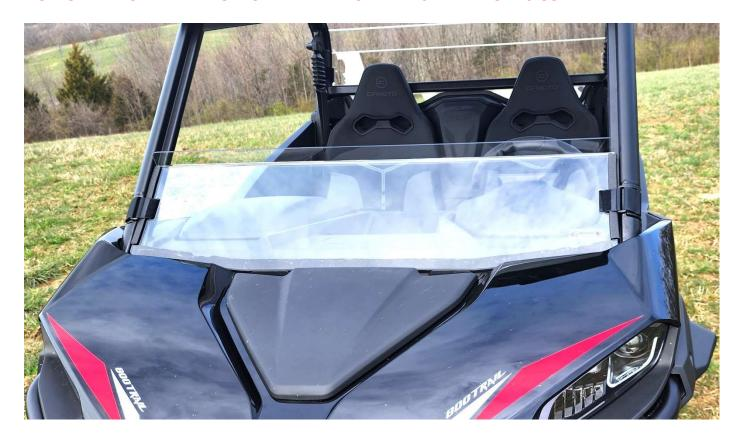
Set windshield in the pro-fit track. Peel back the paper to expose the pre-cut slots. Insert strap through the front of the windshield, wrap around the bar, insert end of strap through plastic buckle and pull tight. Repeat for all remaining straps.
