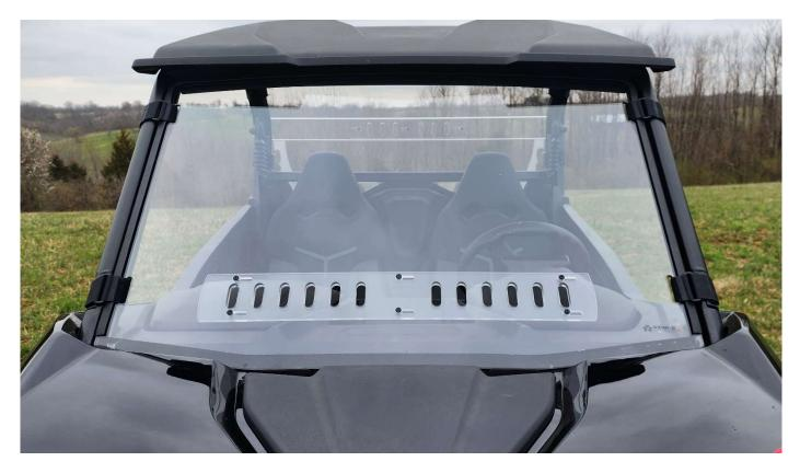
Set windshield in the pro-fit track. Peel back the paper to expose the pre-cut slots. Insert strap through the front of the windshield, wrap around the bar, insert end of strap through plastic buckle and pull tight. Repeat for all remaining straps.
