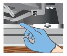
Apply marine grease (or similar) to all moving parts. Remove excess.
