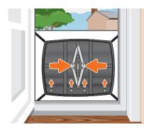
Once the flood threat has passed, loosen the 4 downward pressure bolts and scissor jack, returning the barrier to its unexpanded state.
