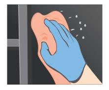
Remove excess moisture from the metal frame using a clean cloth. Examine for damage caused by stress, use or wear and tear, paying particular attention to the operating mechanisms.
