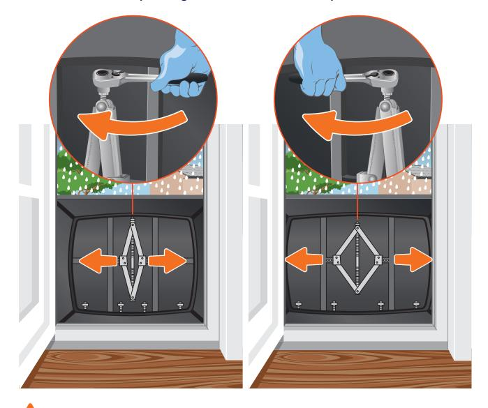
Using excessive force may result in damage to the product or doorway.
