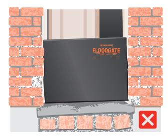
To help achieve an effective seal, walls need to be plumb, parallel with one another and at right angles to a level step/ground. Walls need to be sufficiently strong to cope with the lateral pressure exerted by the barrier.
