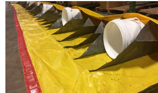
Place objects to raise Water Force to dry out, prior to storage
