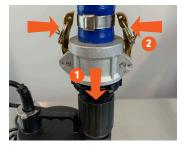
Attach hose fitting on the end of the upper pump fitting and clamp into position
