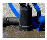
Place pump in low lying area or where potential water issues may happen. Pump will dry to 1/8" and is ok to run dry
