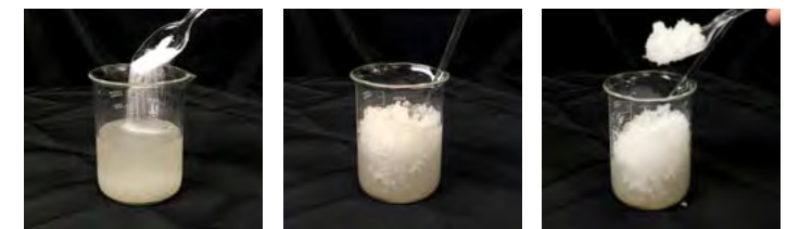
Add Liquid Lock to slurry liquid
