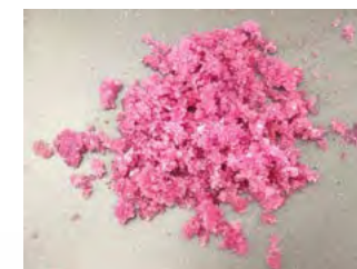
4) Spilled liquid has been neutralized & absorbed
