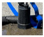
Place pump in low lying area or where potential water issues may happen. Pump will dry to 1/8" and is ok to run dry
