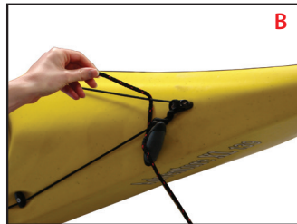
Keeping the rope tight and in place, thread the free end up and through a strong point on the kayak
