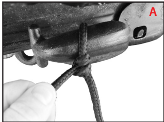
Attach Safety line to vehicle tow ring or other sturdy body part.
