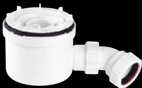
50mm Water Seal Trap Body with 1½" Multifit outlet. Overall height with tile 120mm. Flow rate 42 l/min*
