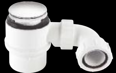
50mm Water Seal Trap with 70mm CP stainless steel mushroom flange. Overall height 95mm
