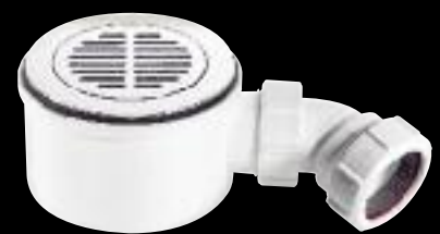
90mm x 50mm Water Seal Trap with 1½" Multifit Outlet and CP brass flange. Overall height 70mm
