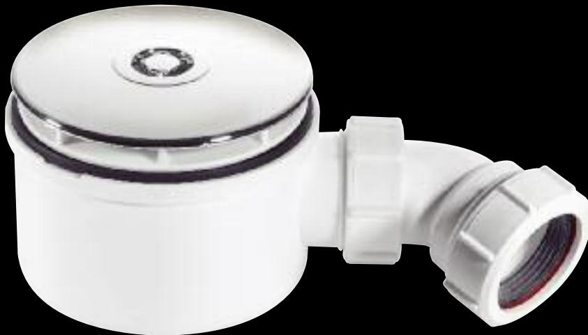
90mm x 50mm Water Seal Trap with 1½" Multifit Outlet and CP plastic flange. Overall height 70mm
