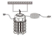
Step 3: Connect each temporary work light. Max. 8pcs 100W in series. Turn on the power (AC 100-277V) and test.
