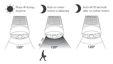
Note: This solar wall light also features photocell, so it will get fully charged during the daytime and release its energy at night.
