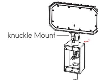
4. Using the wire nuts, connect the wires in the junction box. Connect the ground wire to the green wire; the live wire to the black wire; the neutral wire to the white wire.
