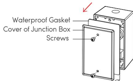
2. Pass the lamp wires through the hole of the junction box.
