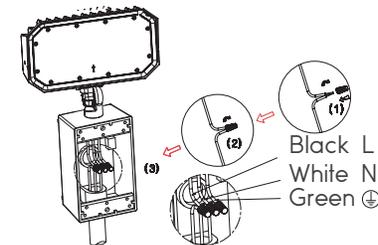
5. Use the screwdriver to screw back on the junction box cover.
