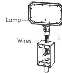
3. Screw the knuckle mount into the junction box.
