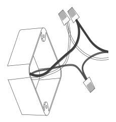
3. Use M4 x 10 screws to connect the lamp body on the junction box. Make sure all the parts are connected firmly.
