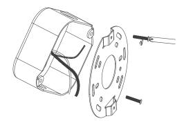
2. Take out wire connectors in attached bags, connect the input wire from fixture with internal wire from the junction box, ground wire to ground wire (L to L, N to N).
