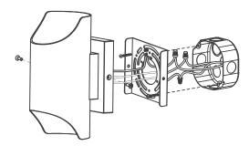
4. The installation is now complete. Fill the gap between the fixture and wall using silicone sealant. Turn the power back on.
