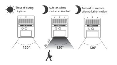
Note: This solar wall light features a photocell, during the day it will charge until full and at night it will release that energy.
