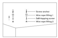
2. Adjust the wire rope to make the panel hang horizontally.
