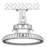
3. Connect wirings in accordance with local connection standard. Make sure the joint protective measures is proper. Connect the green/yellow wire to the ground wire, the brown/black wire to the ACL, the blue/white wire to the ACN. The installation is now complete.
