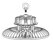
2. Hang the fixture on the ceiling's hook or chain. Be careful not to drop the fixture.
