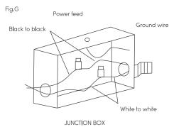
3. After completing the wiring, snap wiring box cover closed (make sure the wires are placed neatly in the junction box).
