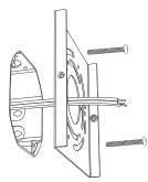
3. Using the wire nuts, connect the wires. Connect the black fixture wire to the black supply wire, the white fixture wire to the white supply wire, and the green wire to the ground wire. Carefully tuck all the wires back into the junction box.
