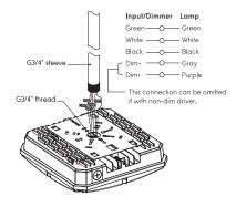
2. Rotate the steeve to make it fixed with lamp. Installation is completed.
