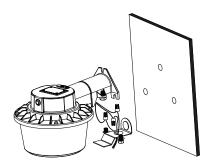
3. Lock the brackets back to body of the light with two screws.
