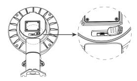
Open the rubber cover to adjust the color temperature.
