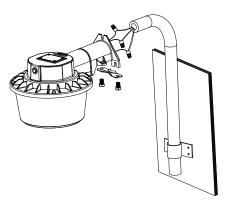
4. At last, lock the bracket to the light with two screws.
