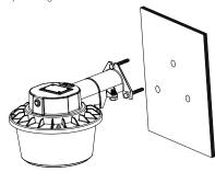
4. At last, lock the light on the wall or wood with three screws.
