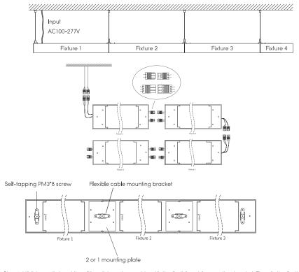
Step 4. Lift fixture 1 first and then lift up fixture 2's one side with the flexible cable mounting bracket. Then fix the flexible bracket in place by using the supplied PM3\*8 screw.
