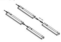
2. Use a lamp connector to connect the lamps.
