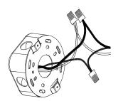
4. Use a screwdriver (not included) to screw in the screws to fix the lamp to the mounting plate and make sure that it's perfectly fixed. Make sure that the wires are not pinched between the mounting plate and the lamp.
