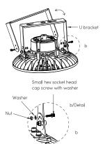
4. Screw the lifting ring on the U bracket. Tighten it using a nut.
