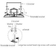
3. Adjust the U bracket's angle. Remove a washer and the nut from the small hex socket head cap screw nut with washer. Pass the screw and the other parts through holes on the U bracket and the rotatable bracket. Tighten the screw using the washer and the nut.
