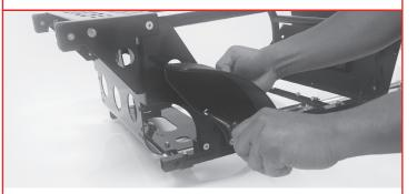
6. Line up the lower hole in the fender with the nut inside of the fender lock. Use a 16mm bolt to secure. Tighten fully and then tighten the bolt from Step 4. 7. Repeat Steps 1-6 for the alternate fender.
