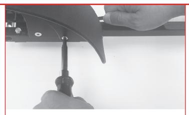
4. Attach the left fender using a 35mm bolt and the nut from Step 3. Pass the bolt through the top hole in the fender from the outside, through the square tube into the nut. Do not fully tighten.
