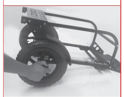
Reinstall the wheels, spacer and axle.
