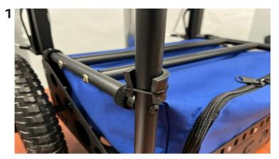
**STEP 2** Align the two halves of the inline bracket around the spacer, insert screw through the bracket from front to back, place nut in back of bracket with the collar of the nut in the hole. Tighten screw with supplied 5mm hex key, make screw only tight enough to hold bracket in place, (if supplied black tube will not slide into bracket it is too tight).
