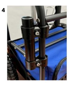
**STEP 5** Assemble 45-degree bracket screw and nut to bracket and place over top of short tube, with the low end of the bracket toward the front of the cart. Slide long tube into bracket with the end of the tube is flush with the front edge of the bracket. Tighten screw so tube is secure. The frame is now complete.
