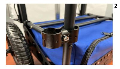
**STEP 2** Align the two halves of the inline bracket around the spacer, insert screw through the bracket from front to back, place nut in back of bracket with the collar of the nut in the hole. Tighten screw with supplied 5mm hex key, make screw only tight enough to hold bracket in place, (if supplied black tube will not slide into bracket it is too tight). Repeat steps 1 & 2 for remaining in line bracket locating it just below the upper front horizontal tube of the cart.
