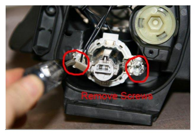
First twist the bulb as shown, then the bulb should Gently pull out
