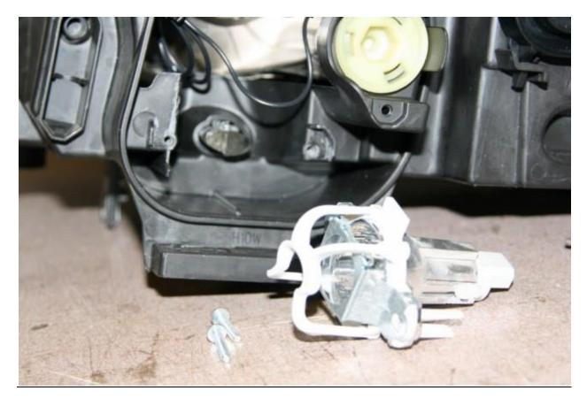
Insert the new LUX LCI Halogen unit and re-insert the screws
