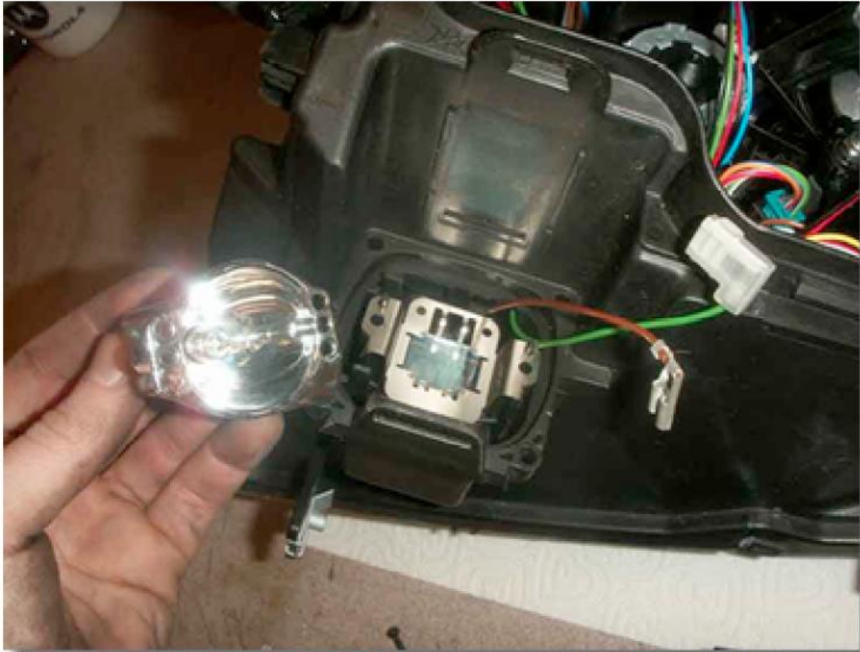
Picture 10. You will now have the OEM bulb and you will see the metal piece holding the clear glass. Remove the metal piece ( and there is a plastic holder attached as well).
