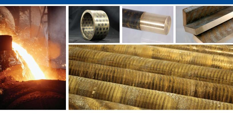
C86300 (SAE 430-B) High Strength Cast Manganese Bronze, has outstanding mechanical properties to withstand the most rigorous industrial requirements. Its high strength and corrosion resistance make it ideal for heavy-duty applications. It outperforms and outlasts general purpose bronzes in the toughest applications.
