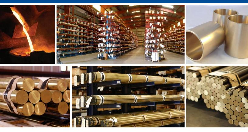
This is a high leaded tin bronze used for high speed and heavy pressure applications where corrosion resistance is necessary. The increased lead content provides added self lubricity within the family of tin bronzes. Excellent machinability at 80%!
