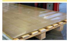
Available in solid bars, hex bars, flats, and plates This lead free alloy maintains a machinability of 30% and posses mechanical properties better than regular brass. Typical uses are in seal glands, nuts, valve stems & seats. Its name 'Naval Brass' stems from its marine application usage such as marine hardware, flanges, baffle plates, and end plates (Discs) for heat exchangers.
