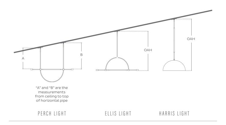
Each of our pendants may be hung from a pitched ceiling of up to 45 degrees. For any pendant with one down rod, please provide the desired overall height (OAH) measurement. The is the total height of the fixture from the ceiling to the bottom of the fixture.
