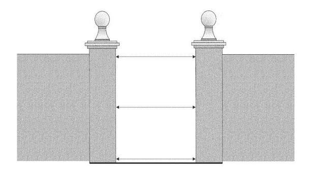
Take the shortest of the three measurements and reduce by 100mm (or 4"). This allows for the hinge (inc pins) and opening gap. The final figure will be the actual width of gate required.
