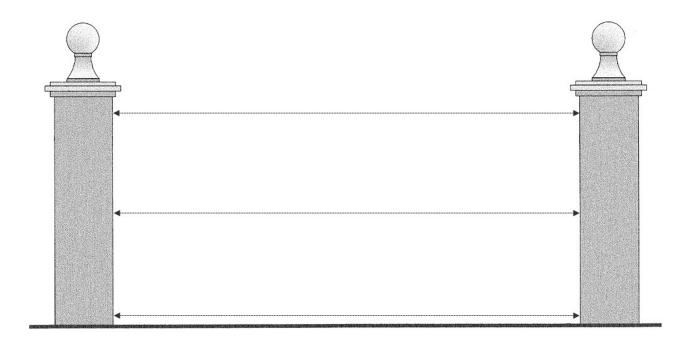
Take the shortest of the three measurements and reduce by 150mm (or 6"). This allows for the hinge (inc pins) and opening gap. The final figure will be the actual width of gate required.
