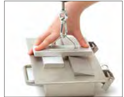
Rare Earth Plate Magnet Pull Test using non-magnetic spacers & 1/8" bar test piece.
