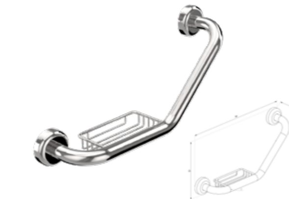
ANGLED GRAB RAIL WITH SOAP DISH NH42 - W - 440 D - 227 P - 106 Ø - 25.4
